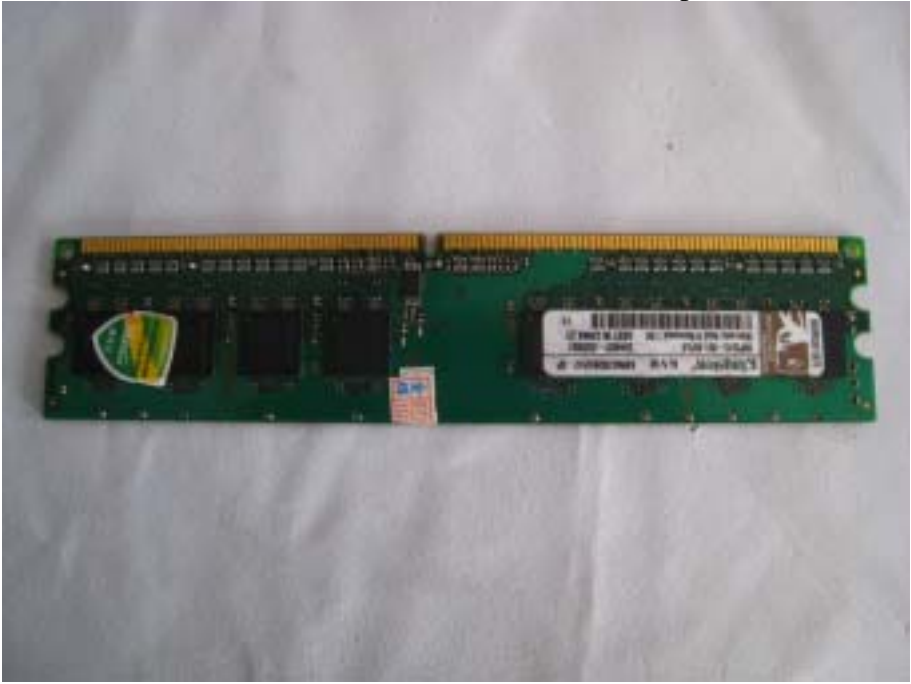
Figure 5 Components Side of the PCB
