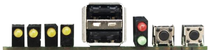
Front I/O card with 2 * USB 2.0, Power & Reset button, Power & HDD LED & 4 * NIC LEDs
